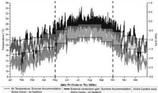
Fig.12: Annual thermal performance of the summer accommodation derived from thermal analysis by using IES programme.
