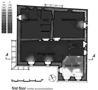
Fig 8: Winter accommodation daylight analysis by using Ecotect software
