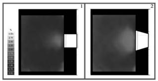
*Fig. 7: 1. Room without splayed reveal window in plan (Av.DF: 1.10%), 2. Room with splayed reveal window in plan (Av.DF: 1.30%). Daylight simulation by using Ecotect software.*
