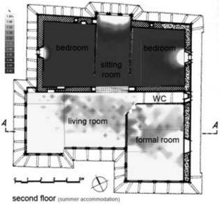
Fig.10: Summer accommodation daylight analysis by using Ecotect
